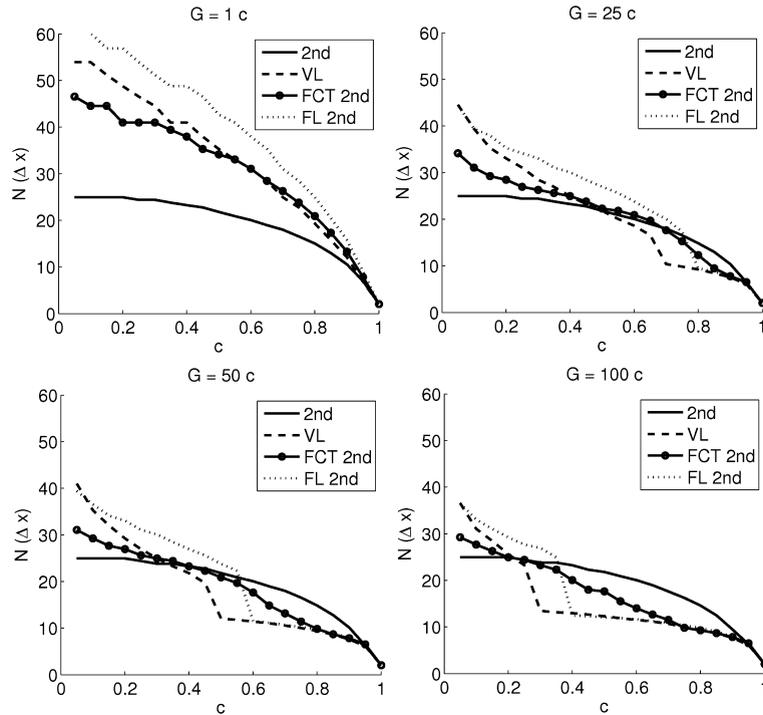
**Fig. 2.** Numerically calculated effective resolution, in terms of  $N\Delta x$ , against Courant number  $c$ , for the second-order forward-in-time (2nd), van Leer (VL), flux-corrected transport (FCT 2nd) and the universal flux-limited (FL 2nd) schemes. The results are shown for different length simulations; 1 time step (top left), 25 time steps (top right), 50 time steps (bottom left), and 100 time steps (bottom right).
