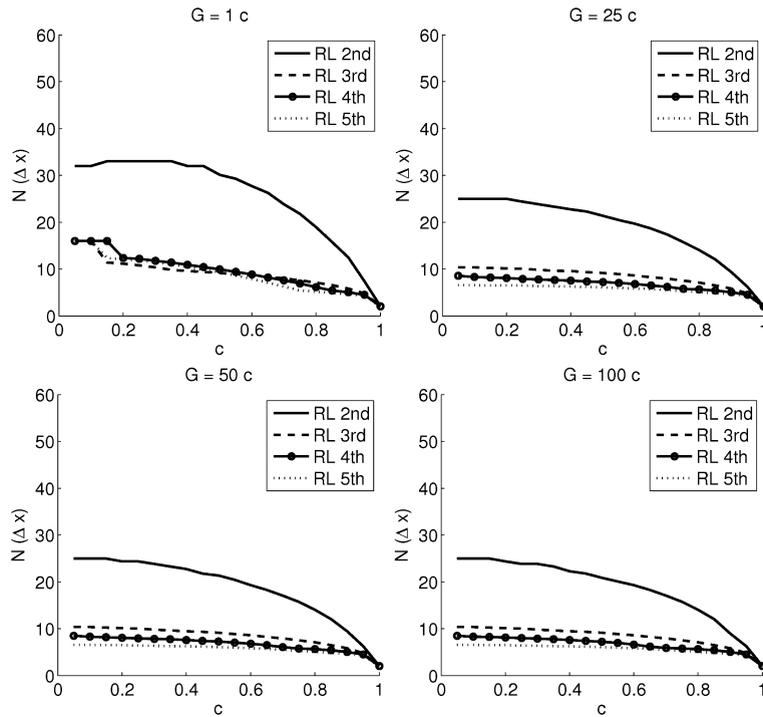
**Fig. 4.** Numerically calculated effective resolution, in terms of  $N\Delta x$ , against Courant number  $c$ , for the relaxed-limiter used with the second (RL 2nd), third (RL 3rd), fourth (RL 4th) and fifth-order (RL 5th) forward-in-time schemes. The results are shown for different length simulations; 1 time step (top left), 25 time steps (top right), 50 time steps (bottom left), and 100 time steps (bottom right).
