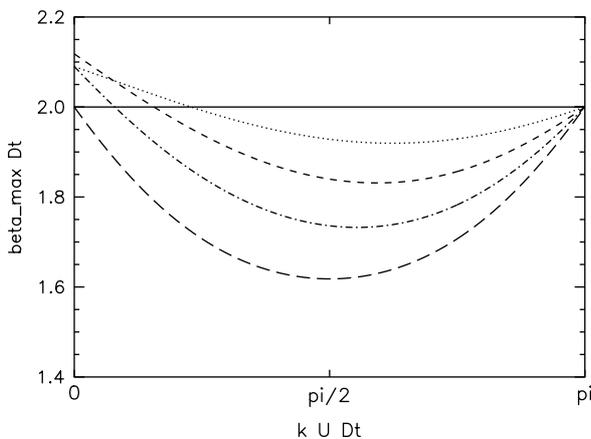
Figure 1. The maximum value  $\beta_{\max} \Delta t$  for conditional stability, as a function of the dimensional parameter  $kU \Delta t$  (see text for explanation), for a diffusive process coupled to the dynamics with  $\omega^* \Delta t = 1$  for different choices  $\omega = \omega^*$  (solid line),  $\omega = 0.75 \omega^*$  (dots),  $\omega = 0.5 \omega^*$  (short dashes),  $\omega = 0.25 \omega^*$  (dash dot),  $\omega = 0$  (long dashes).
