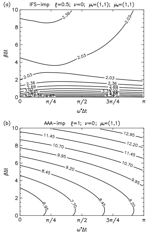
Figure 5. The ratio  $|F_A^+ / F_{\text{forced}}^{\text{exact}}|$  of the amplitude of the approximate forced response, calculated (a) with (32) and (b) with (34), to the exact one (Table 3).
