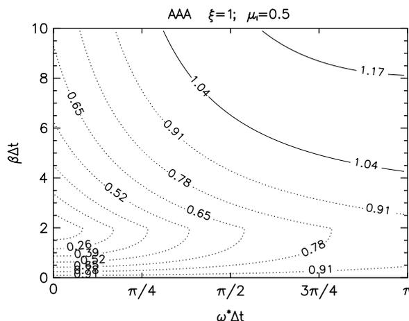
Figure 4. The amplification factor  $|A|$  of the scheme  $\phi_{0.5}^I \mapsto \mathcal{D}^{\text{exp}} \mapsto \mathcal{D}^{\text{imp}}$ .
