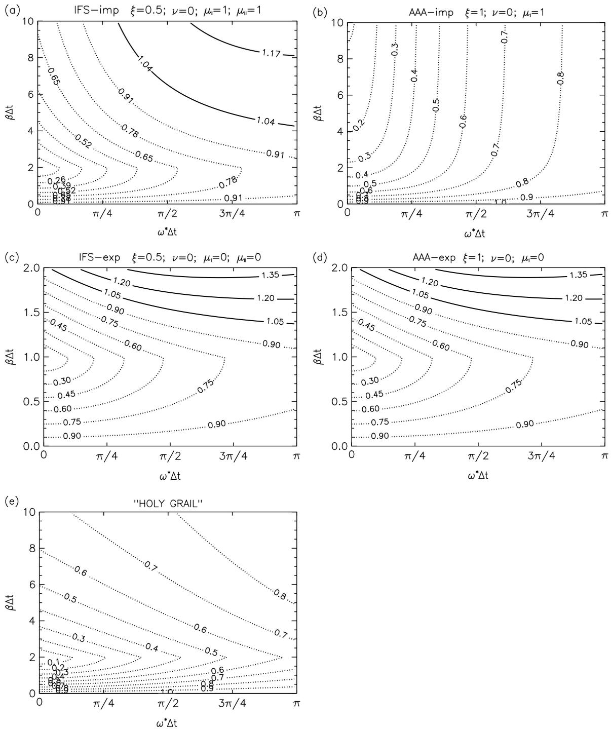
Figure 2. The amplification factor  $|A|$  derived from Von Neumann's method as a function of the dynamics discretization, parametrized by  $\omega^* \Delta t$ , and the amount of diffusion expressed by  $\beta \Delta t$ , for the four schemes presented in Table VI and for the 'holy grail' solution.
